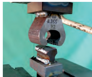
After testing, failure through deformation
